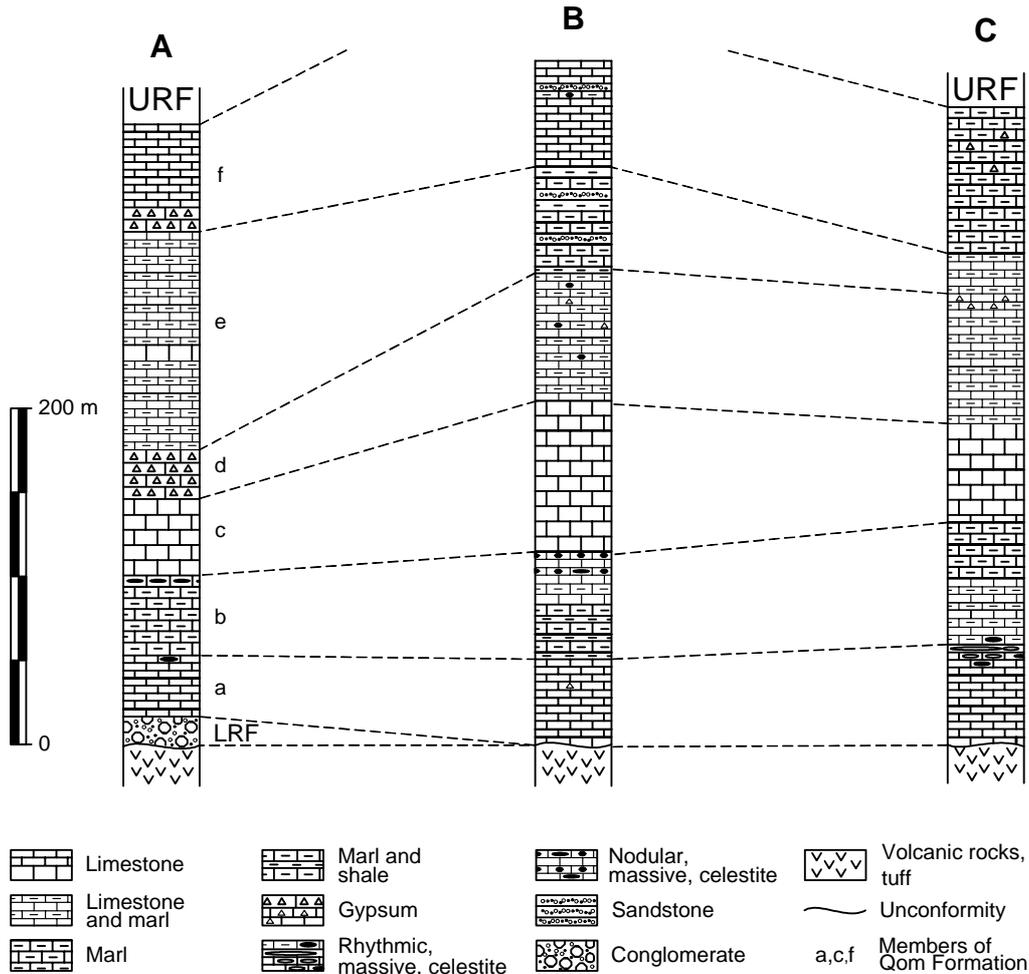
Fig.2 Stratigraphic columns section of the Davazdah-Emam (A), west Siah-Kuh (B) and Molkabad ore deposit (C). For profiles locations see Fig. 1.
